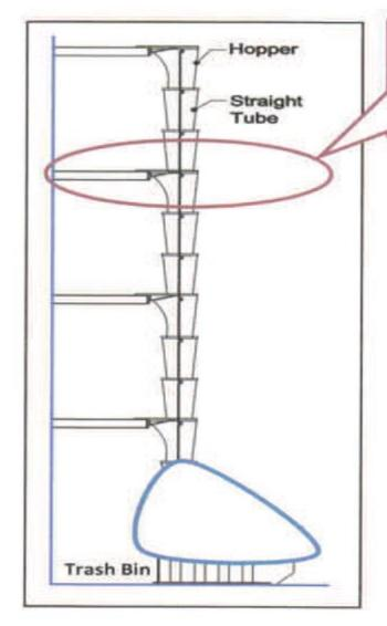
Installing debris disposal ducts on each floor
