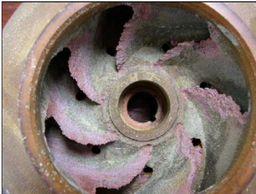
Figure 0-8— Erosion due to Cavitation (Mahdi, n.d.)
