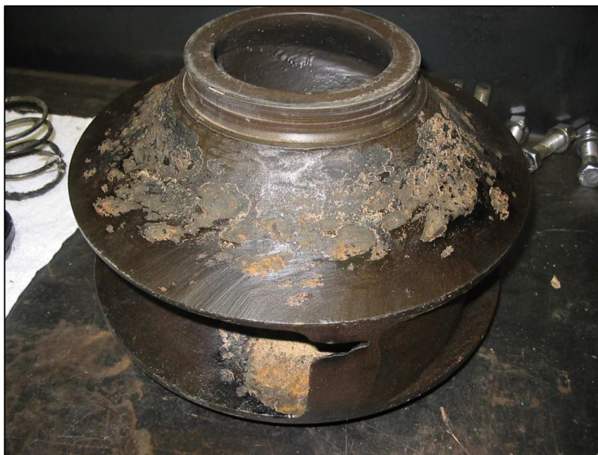
Figure 0-9— Erosion on Pump Impeller (PES Solutions, 2015)
